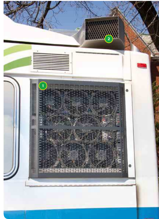
The low-voltage electric ventilator system (1) was installed on the outside of the radiator on an STM hybrid bus and an STM standard bus. A section for cooling the hybrid transmission fluid (2) was added on the roof of the hybrid bus.
